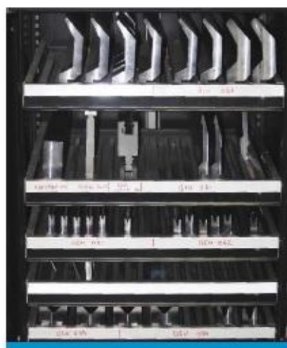
A Wila storage cabinet protects tooling which is offered in segmented lengths for single operator loading and unloading.
