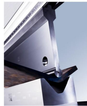
Figure 15. Photograph shows a heavy plate bending application. While often overlooked, the need for hardened tooling is greatest when bending thick abrasive, plate materials.
