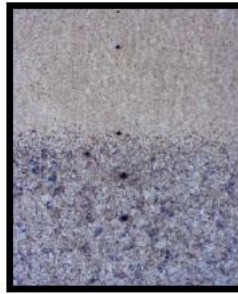
Figure 8. Magnification of 100x shows the transition from the CNC DeePhardened® area (light color) to the base material
