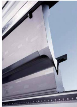
Figure 14. Photograph shows a precision air bending application where the slightest inaccuracy along the Ty axis can result in an angular error of several degrees.
